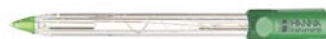
HI10533 Triple ceramic, double junction, glass body, refillable pH electrode with conical tip and temperature sensor Recommended for fats, creams, soil and low conductivity samples
