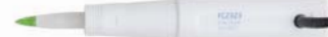
FC2323 Open viscolene reference electrolyte, double junction, PVDF body pH electrode with conical tip and temperature sensor Recommended for meat applications with use of optional FC098 20 mm (0.8") or FC099 35 mm (1.4") stainless steel blade
