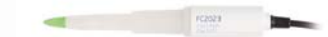
FC2023 Open viscolene reference electrolyte, double junction, PVDF body pH electrode with conical tip and temperature sensor Recommended for dairy analysis including cheese, yogurt, and other semi-solids
