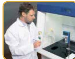
Tracer gas containment test
