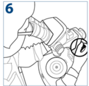
6 Rotate the focusing knob to bring the specimen into focus
