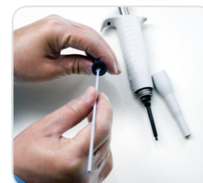
Proline® Plus pipettes have only three parts that need cleaning and maintenance.
