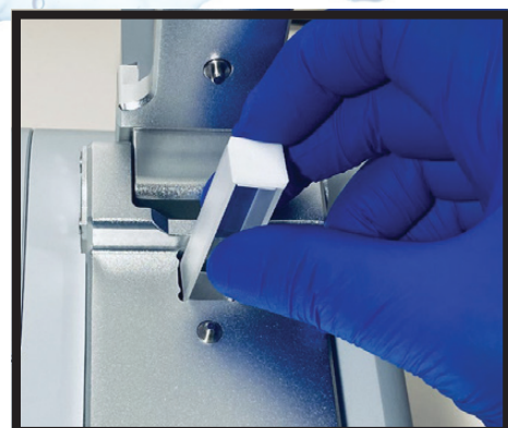
Cuvette port for OD600 readings
