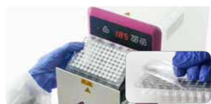
Figure 2: Random Access Sealing Procedure using the 4s3™ Semi-Automatic Sheet Heat Sealer (4ti-0655)
